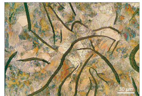
Brightfield image of gray cast iron with GJL flake graphite. Courtesy: University of Applied Sciences, Aalen, Germany.
