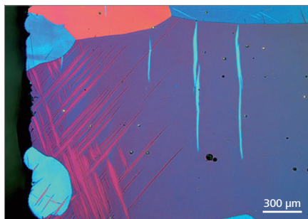
Polarized image of zinc with deformation twins. Courtesy: University of Applied Sciences, Aalen, Germany.
