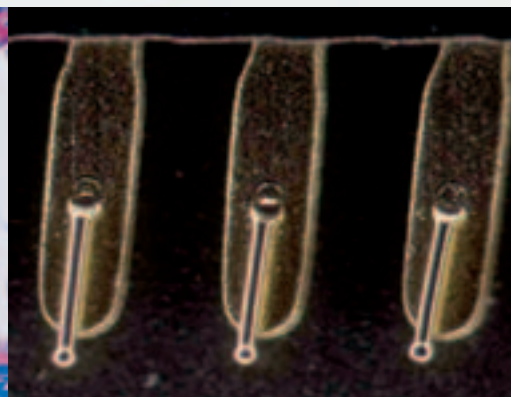
Semi-conductor element. Reflected light-darkfield. Objective: PlanApo S 1.5x Magnification: 125x*
